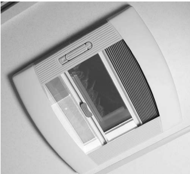
Thermal roof bonnet in bedroom
